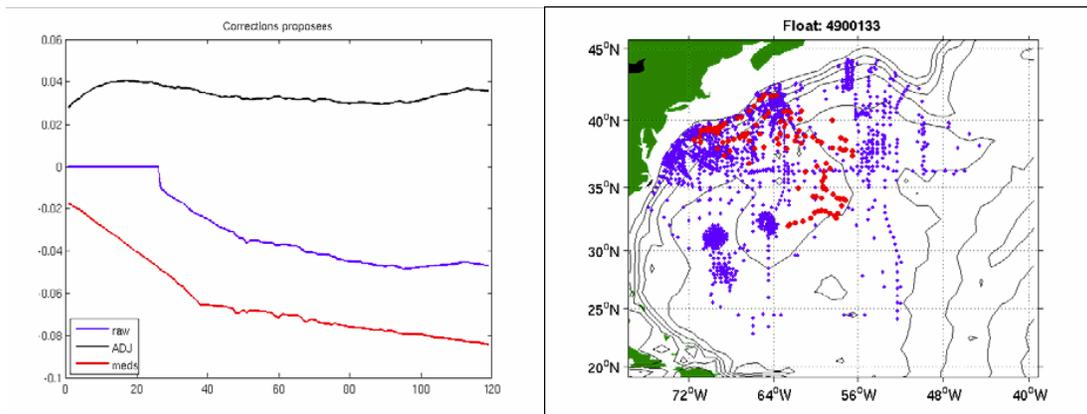
**Figure 2.** Salinity corrections for float 4900133. Correction applied by Meds and used to generate the PSAL\_ADJUSTED fields (red) – Correction to apply on the PSAL data estimated from the statistical method used at Coriolis (blue) – Correction to apply on the PSAL\_ADJUSTED data estimated from the statistical method used at Coriolis (black).
