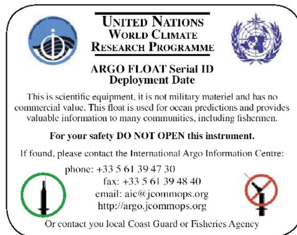
A new Argo label has been produced by Scripps. It is lighter (so that it will not affect float ballasting if the sticker is lost during its mission) and distributed to float manufacturers.
