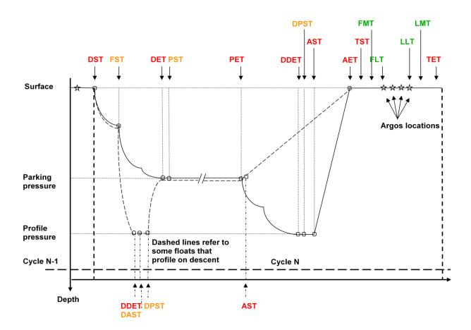
She noted that this diagram is accurate for Argos floats, but not for Iridium/GPS floats. Below is a more accurate diagram of Iridium floats on the surface.
