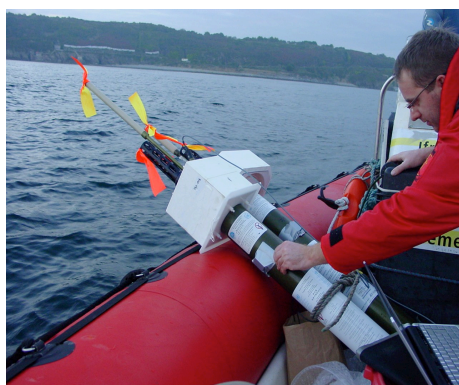
Arvor fitted with Argos3 satellite transmission during tests at sea in October 2010
