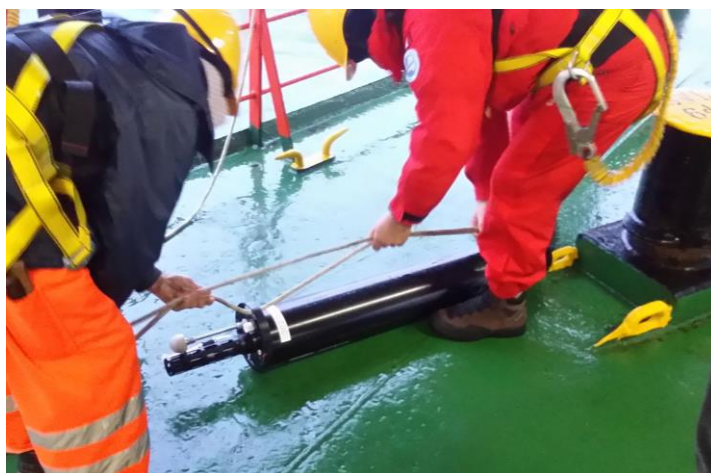
Figure 3. A Nova float ready to be deployed on R/V Italica in January 2016.
