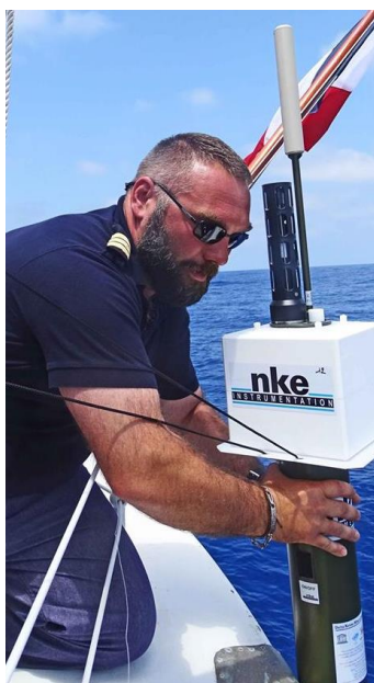
Figure 1. Arvor-I float being deployed in the Tyrrhenian Sea by the French Navy in June 2016.
