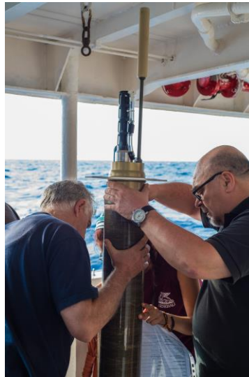
Figure 2. Deep Arvor float (WMO 6903200) before deployment on the R/V Aegaeo on 8 June 2016.
