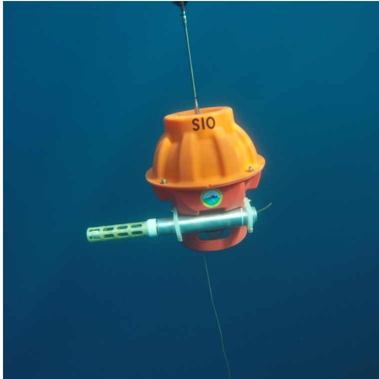
A Deep SOLO float descends from the sea surface off San Diego. The 33 cm diameter spherical glass pressure housing is inside the protective hardhat. The Iridium/GPS antenna, SBE-61 CTD and passive “bottom finder” wire can all be seen. The float’s pancake bladder is inside the bottom cowling, behind the CTD. (Photo by SIO Instrument Development Group)
