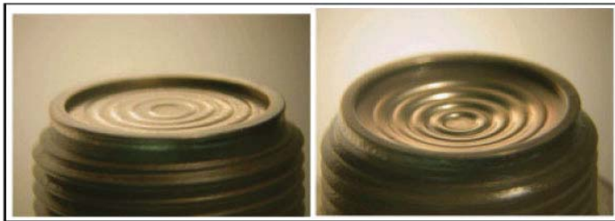
Figure 2. Photographs of the upper end of a normal Druck pressure sensor (left) and one with a deformed titanium diaphragm, indicative of the microleak problem (right).
