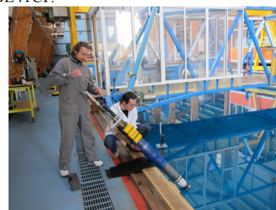
Photo 3: Prototype of deep Arvor during tests at Ifremer pool
