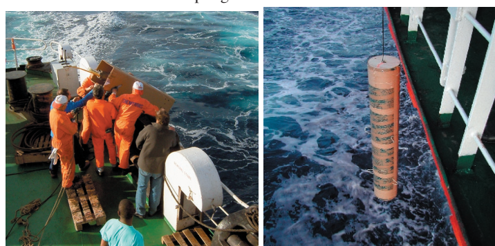
Fig 1 Left. Release of a PROVOR in its VOS deployment box from the aft deck of LNG/LPG carrier Annabella in the southern Ionian Sea (Photo courtesy of A. Cruzado). Right. APEX float in its cylindrical VOS box about to be deployed in the Levantine Sea from container ship Britain Star (Photo courtesy of I. Gertman).
