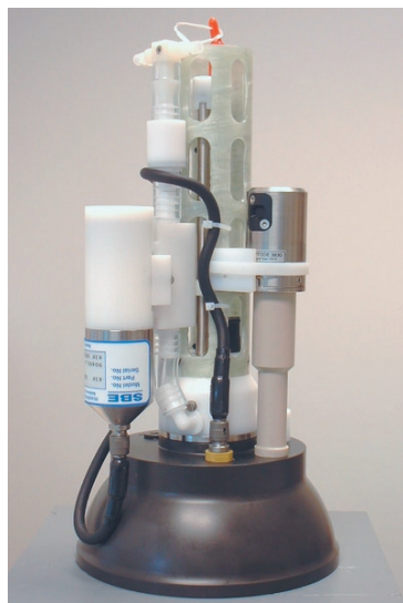
Fig. 1: Photo of the top cap of a profiling float with the two most advanced oceanographic oxygen sensors installed side by side: Seabird Inc. electrochemical sensor on the left, Aanderaa optode sensor on the right. Field results from such dual-oxygen-sensor floats are already available.
