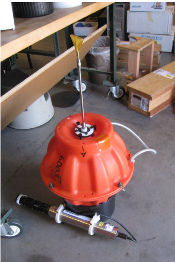
Deep SOLO with externally-mounted SBE-61 CTD
