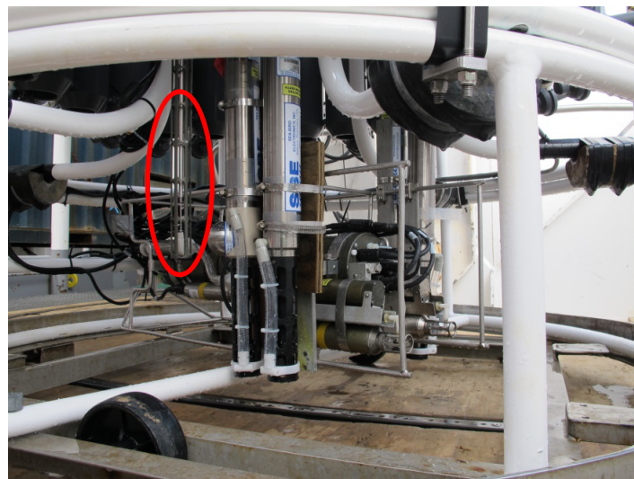
SBE 35 reference thermometer was also mounted.
