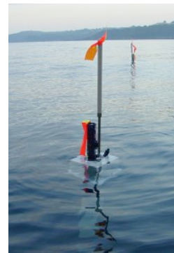
Arvor fitted with Argos3 satellite transmission during tests at sea in October 2010
