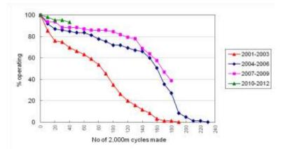
Figure 4. Number of (normalised) cycles made by UK Apex floats deployed in 2001-2003, 2004-2006, 2007-2009 and 2010-2012.
