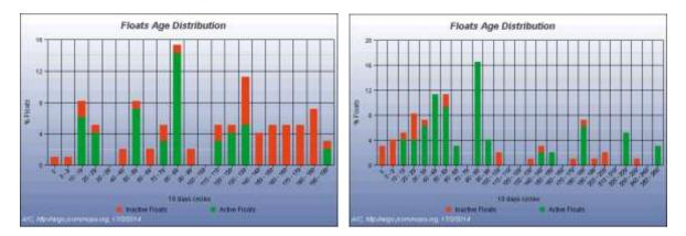
Figure 5. Number of cycles made by UK Apex floats deployed since 2007 with (left) alkaline and (right) lithium batteries. Note the horizontal scales are different.
