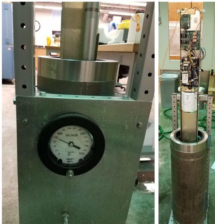
Figure 5: This pressure test vessel (PTV) was custom designed to subject the lower end-cap assembly to high pressure water while simultaneously allowing access to the inside of the float.
