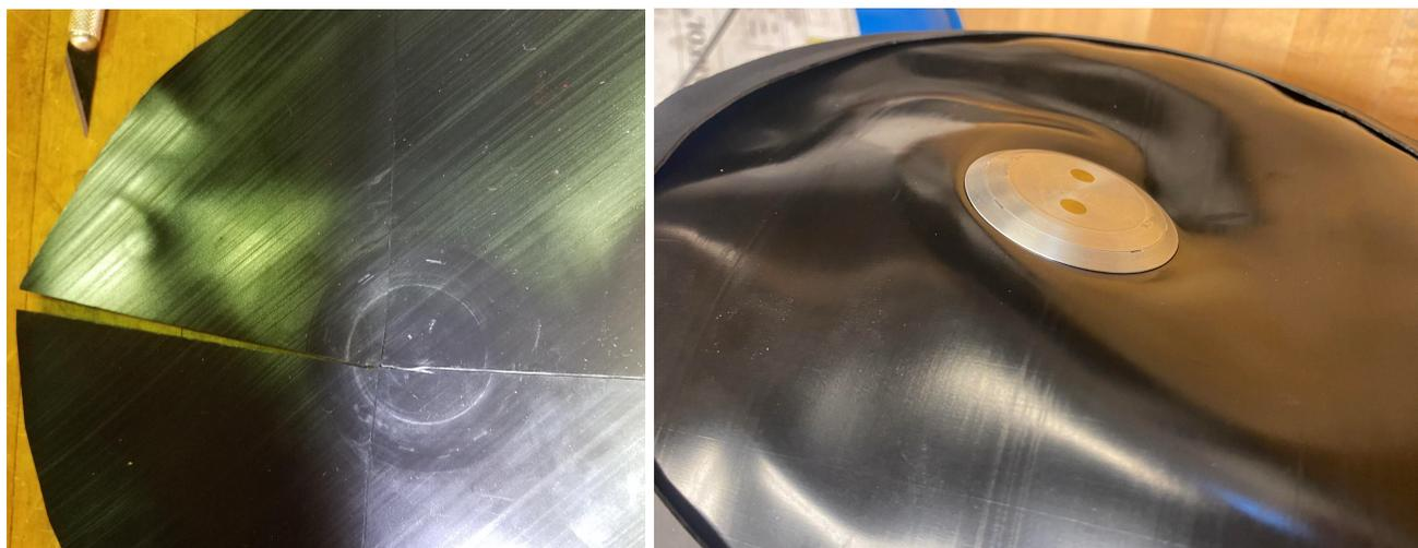
Figure 8: **ApfId 18340 Bladder Section:** (left) The inner surface of the outer wall of the air bladder is marked by linear striations with a median transverse roughness (Ra) measured to be  $16\mu\text{m}$ . (right) The inner surface of the inner wall of the air bladder is smooth and shiny with only a few striations. The median roughness was measured to be  $12\mu\text{m}$ .
