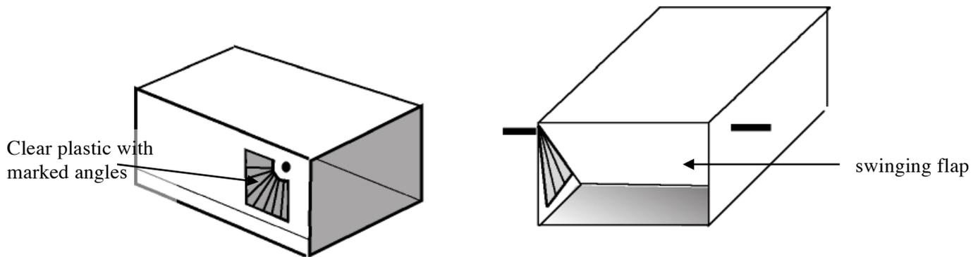
**Observe:** Hold the box so it faces into the wind. Measure the angle of the flap. Use the table to work out the wind speed
