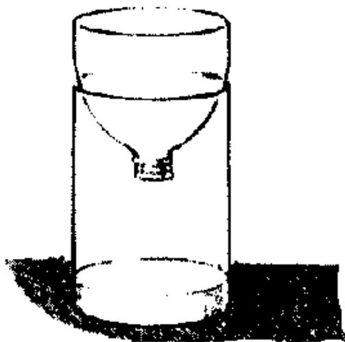
Cut the top off the bottle just below the shoulder. Turn the top upside down to make a funnel. Push this back inside the cut off rim of the bottle.
