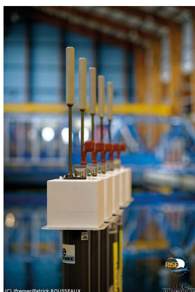
New RBR CTD mounted on the head of the Arvor float (left) and deep-Arvor prototype equipped with 3 CTDS: RBR, SBE41 and SBE61 (right).
