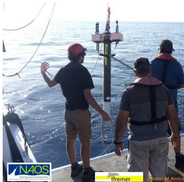
New RBR CTD mounted on the head of the Arvor float (left) and deep-Arvor prototype equipped with 3 CTDS: RBR, SBE41 and SBE61 (right).
