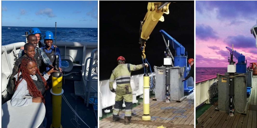
Figure 2: Recent deployments of UK floats: Students from the @oceanx Young Explorers Program deploy a UK Argo float from OceanXplorer as part of the OceanX and OceanQuest “Around Africa” expedition, WMO 1901930, 02/03/25 (left); APEX SBE, WMO 7902225, before deployment from RRS James Cook. Brazil Basin, 19/01/25 (centre, A. Rochner, Met Office); CTS5 Jumbo, WMO 6990670, before deployment from RRS James Cook. Brazil Basin, 19/01/25 (right, A. Rochner, Met Office).
