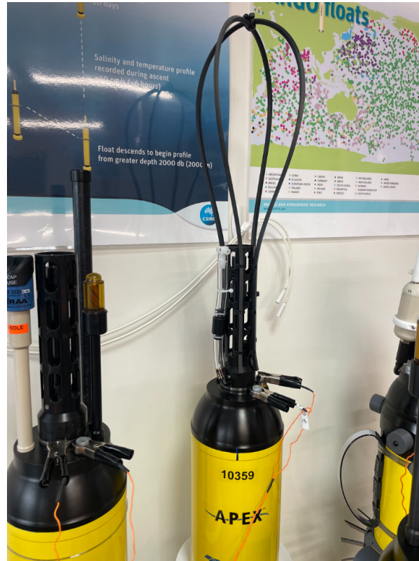
Figure 6: Pole type ice guard (left) and eggbeater type ice guard (right) on TWR APEX APF11 floats.
